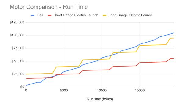
Here, we see that overtime, both a short and long range launch cost less to operate. The large jumps represent purchasing new gas motors or new batteries.
